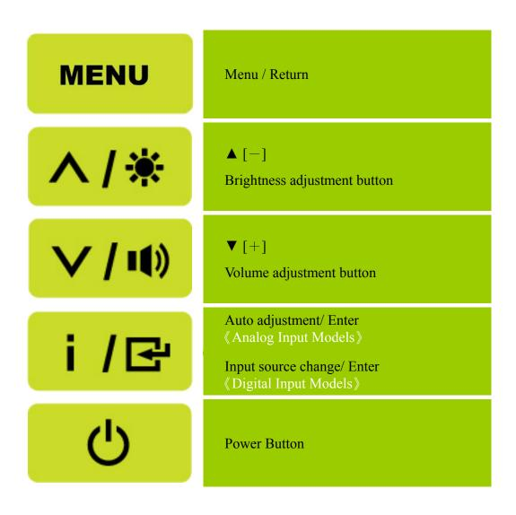
Figure.5. Control Panel Buttons
